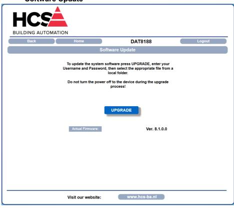
This section allows to update the versions of the firmware or web server and is used in case of necessity. To execute the update click on the button "Upgrade"; the system will open a pop-up window where to insert the credentials to proceed with the update. Contact the Technical Assistance service for information about the procedure to follow. The parameter "Actual Firmware" shows the firmware version loaded on the device.
