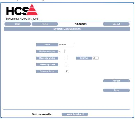
Name: allows to visualize and set the parameter NetBios Name of the device; this parameter is a string and is visualized beside the IP address in the software Dev9k; it can also be used in the software that implement the use of this data.
