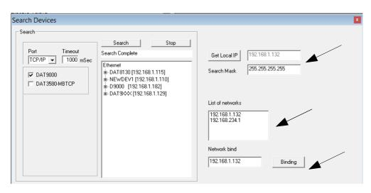
Make sure the IP identified is used in the Network which the device is connected to.
