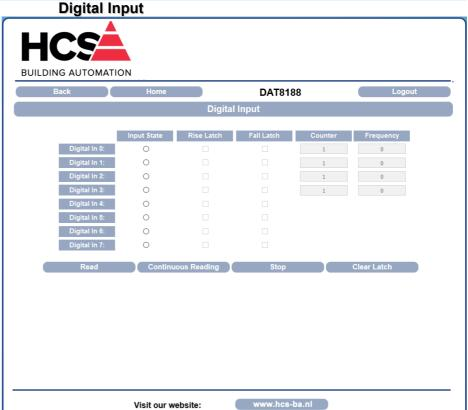
This section allows to visualize the state of the digital inputs and the latchs. Each row is related to each input. To execute a single reading click the button "Read", To execute a continuous reading click the button "Continuos Reading". To stop the reading click the button "Stop". The columns are divided as follows.
