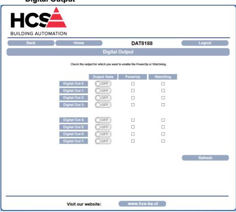
This section allows to visualize and drive the digital outputs. Each row is referred to one output. To execute the update of the page click "Refresh". The columns are divided as follow.
