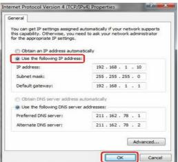
Now the device of DAT8000 series is searchable and the user can change its IP with the desired one. It must be different from the other ones in the network (right click  $\rightarrow$  Set IP address).
