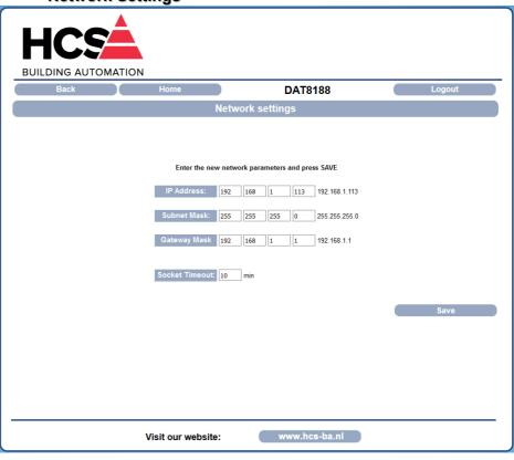
IP Address: allows to visualize and set the unique IP address of the device in the network in use.
